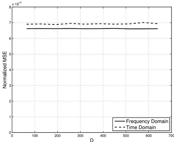
Fig. 4. NMSE of the estimated CSI in stage I for various values of  $D$  when  $L = 64$ ,  $M = 6$ ,  $P = 3$ , and  $\text{SNR} = 10$  dB.
