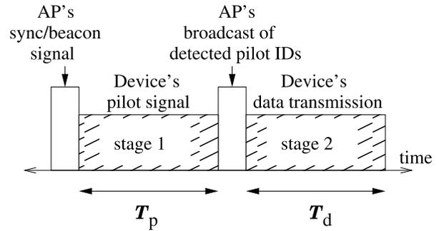
Fig. 2. Illustration of two-stage (uplink) access scheme with the AP's synchronous signal that initiates uplink access by devices.
