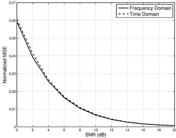
Fig. 3. NMSE of the estimated CSI in stage I for various SNRs when  $L = 64$ ,  $D = 320$ ,  $M = 6$ , and  $P = 3$ .
