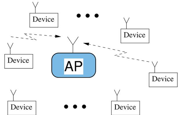
Fig. 1. System model with an AP (or gateway) and multiple devices where a subset of devices are active to transmit their data.
