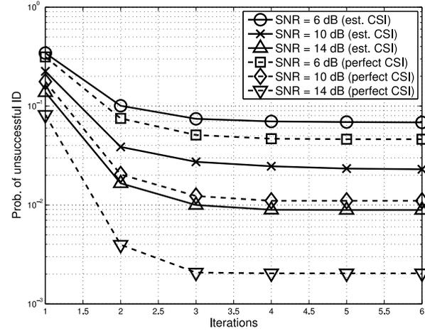
Fig. 7. Performance improvement of the EM algorithm over iterations in terms of the probability of unsuccessful identification when  $L = 64$ ,  $M = 6$ ,  $P = 3$ , and  $Q = 3$ .
