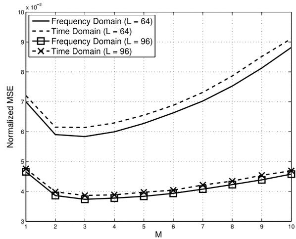
Fig. 5. NMSE of the estimated CSI in stage I for various values of  $M$  when  $L \in \{64, 96\}$ ,  $D = 320$ ,  $P = 3$ , and  $\text{SNR} = 10$  dB.
