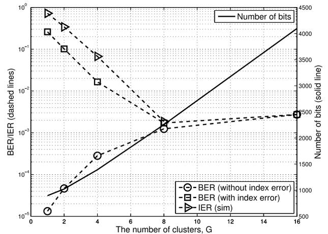
Fig. 7. Performance of OFDM-IM-TD in terms of IER and coded BER for different values of  $G$  when  $B = 2048$ ,  $K = 16$ ,  $Q = 8$ ,  $M = 4$ , and  $\frac{E_b}{N_0} = 6$  dB.
