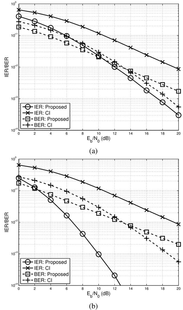
Fig. 3. IER and BER in terms of  $\frac{E_b}{N_0}$  when  $N = 4$ ,  $Q = 2$ , and  $M = 4$ : (a)  $G = 1$ ; (b)  $G = 2$ .
