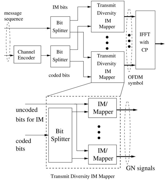
Fig. 1. An illustration of the transmitter for coded OFDM-IM with a transmit diversity scheme.
