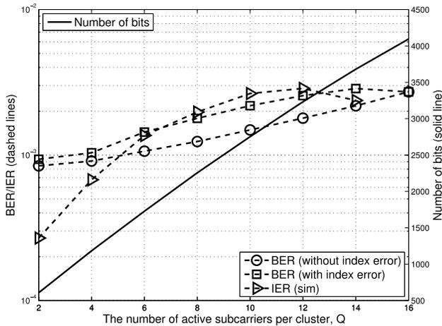
Fig. 6. Performance of OFDM-IM-TD in terms of IER and coded BER for different values of  $Q$  when  $B = 2048$ ,  $K = 16$ ,  $G = 8$ ,  $M = 4$ , and  $\frac{E_b}{N_0} = 6$  dB.
