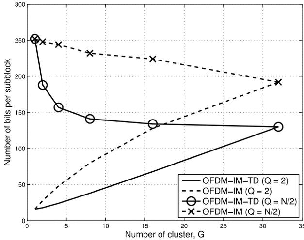
Fig. 2. The number of bits per subblock for different values of  $G$  when  $L = 128$  and  $M = 4$ .
