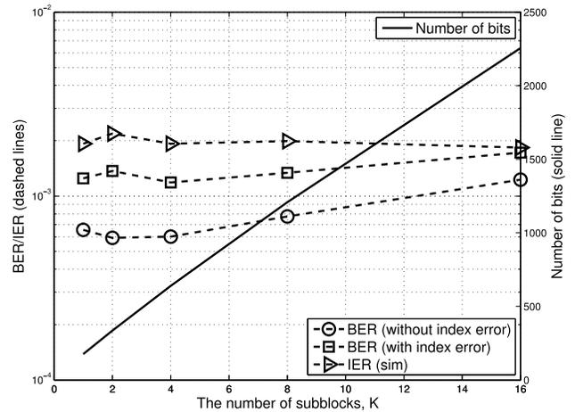
Fig. 8. Performance of OFDM-IM-TD in terms of IER and coded BER for different values of  $K$  when  $B = 2048$ ,  $G = 8$ ,  $Q = 8$ ,  $M = 4$ , and  $\frac{E_b}{N_0} = 6$  dB.
