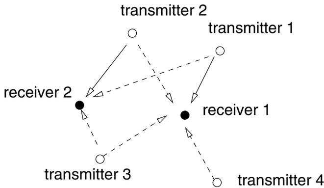
Fig. 1. An example of the system with  $K = 4$  (solid lines represent the desired signals, while dashed lines represents undesired signals).
