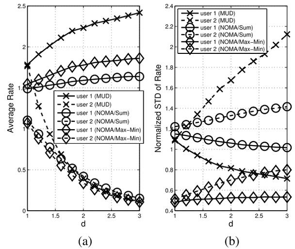
Fig. 2. Performances of the three PFS schemes for different values of  $d$  when  $P_T = 10$  dB and  $\nu = 0.9$ : (a) transmission rates; (b) normalized STD of rates.
