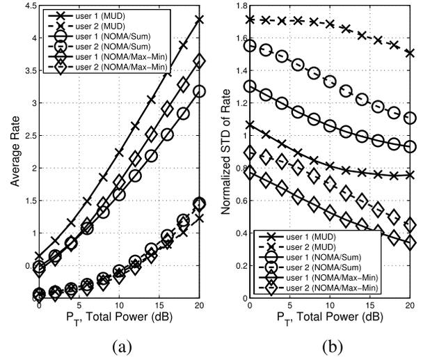
Fig. 1. Performances of the three PFS schemes for different values of the total power,  $P_T$  when  $d = 2$  and  $\nu = 0.9$ : (a) transmission rates; (b) normalized STD of rates.
