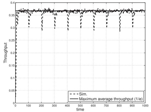
Fig. 4. Throughput when the access probability,  $p$ , is periodically updated between 0.1 and 0.05 every 100 stages with  $K = 1000$ .
