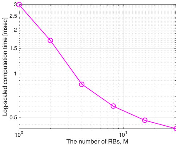
Fig. 4. Computation time over the number of RBs with  $K_A(m) = 3$ .
