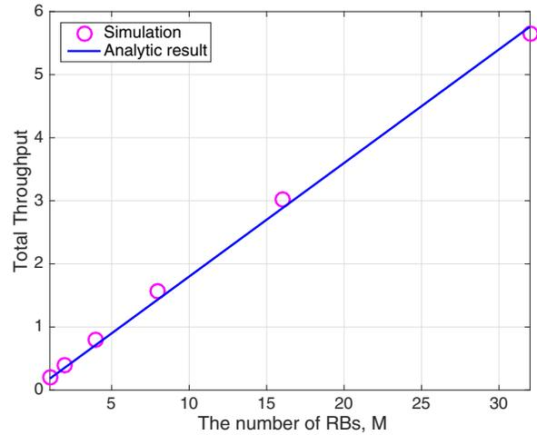
Fig. 2. Total throughput versus the number of RBs with  $p_a = 0.1$
