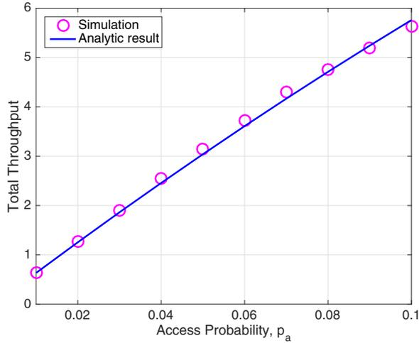
Fig. 3. Total throughput versus access probability with  $M = 32$
