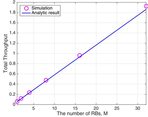
Fig. 1. Total throughput versus the number of RBs with  $p_a = 0.03$
